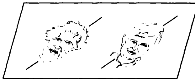
Fig. 11 Passive strain markers (images of John Ramsay and Martin Huber) on the side of a Plasticene block of high viscosity deformed by a plane stress field of unknown orientation. The base of the block remained stable throughout the deformation. The finite stretch S_1 = 1.14 and the inclination of the greatest axis of the strain ellipsoid with respect to the base of the deformed block is \theta = 76^\circ . These data are sufficient to infer from the nomogram of Fig. 9 that the major axis of stress causing the deformation was oriented at 40^\circ to the normal to the base of the block. The same inclination of the stress axis can be determined, using Fig. 10, from the fractional change in orthogonal thickness of 0.96 and the rotation of the edge of the block, which was initially at 90^\circ to the reference plane, and is now at 75^\circ .
